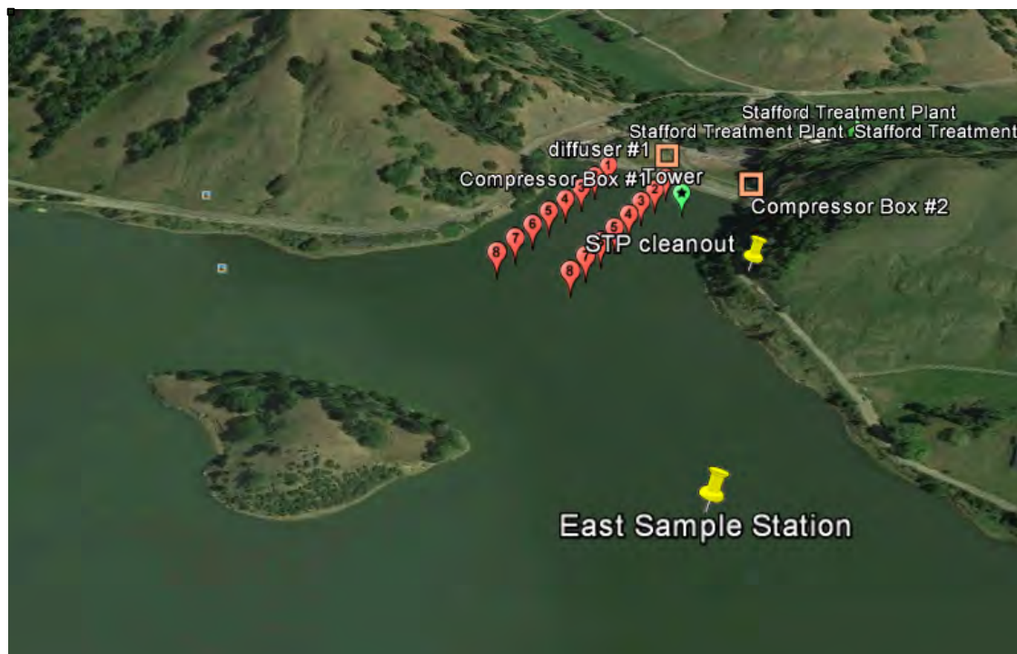
Figure 8 Stafford Lake Existing Keeton Aeration System
