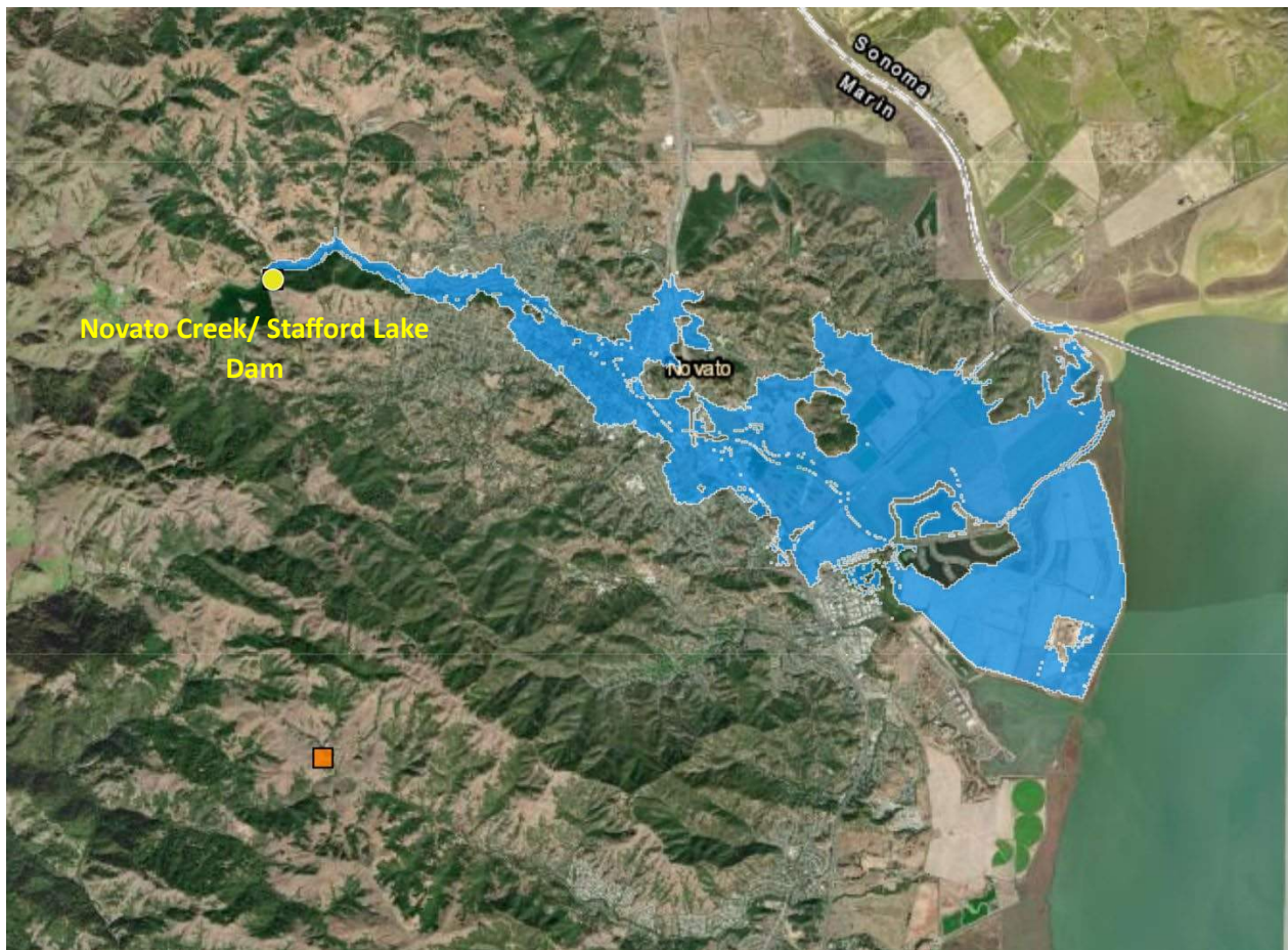
Figure 369: City of Novato - Nonato Creek Dam Inundation Impact Source: California Department of Water Resources, DSOD
