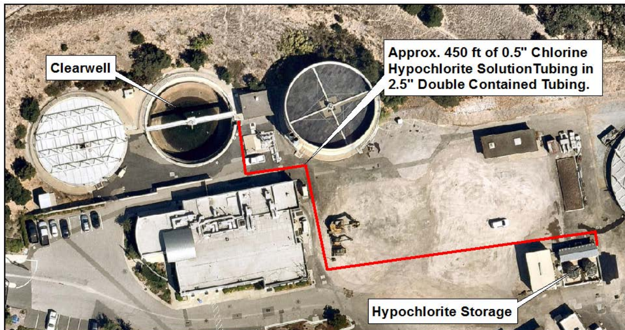
Figure 3-4: Chlorine Injection at Clearwell
