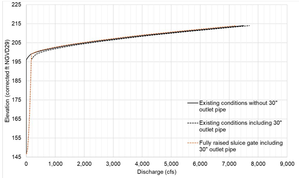
Figure 12. Elevation-discharge curves for existing and proposed spillway
