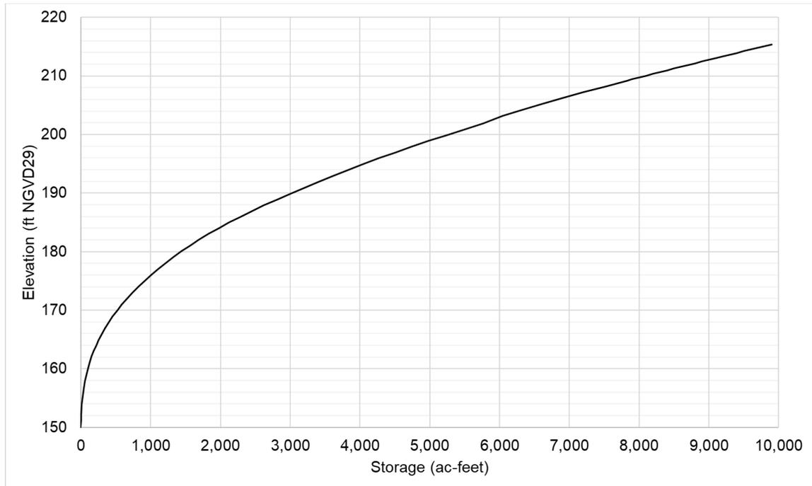
Figure 11. Stage-storage curve for existing spillway conditions
