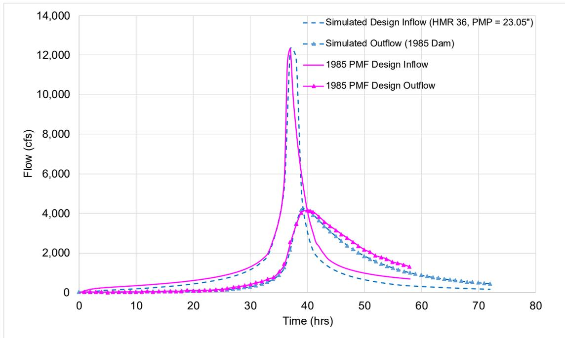
Figure 4: Comparison of 1985 design report PMF inflow/outflow hydrograph and simulated HMS PMF inflow/outflow hydrograph
