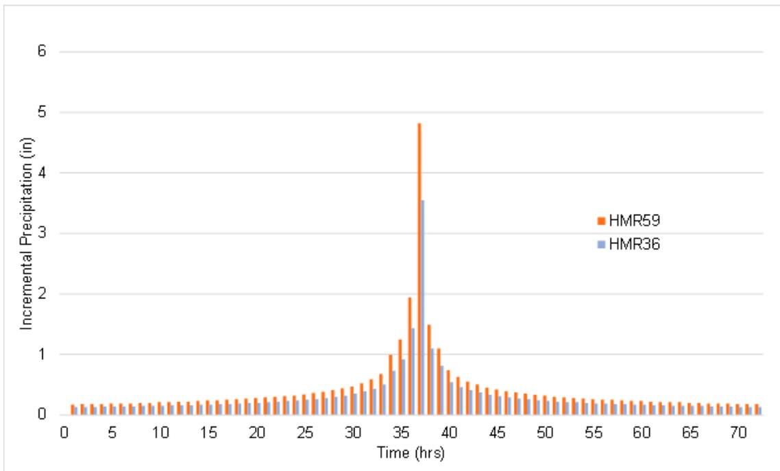
Figure 3: Comparison of General Storm (72-hour) PMP hyetograph under HMR 36 and HMR 59
