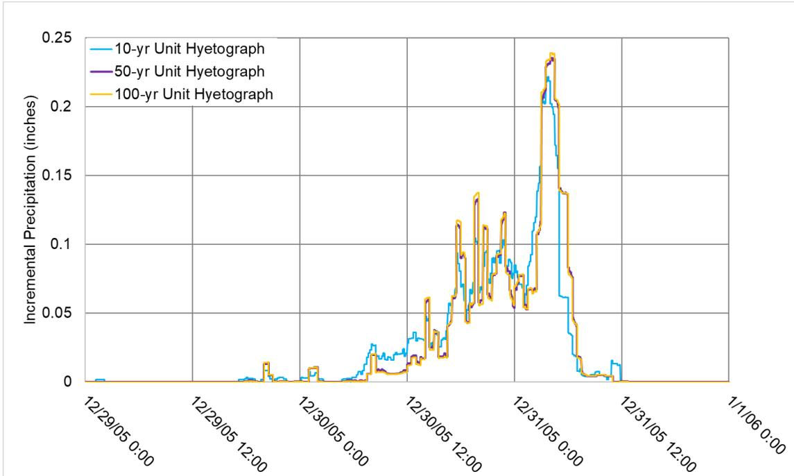
Figure 6. Unit Hyetograph Comparison of 10-, 50, and 100-year design events for Subbasin W1710
