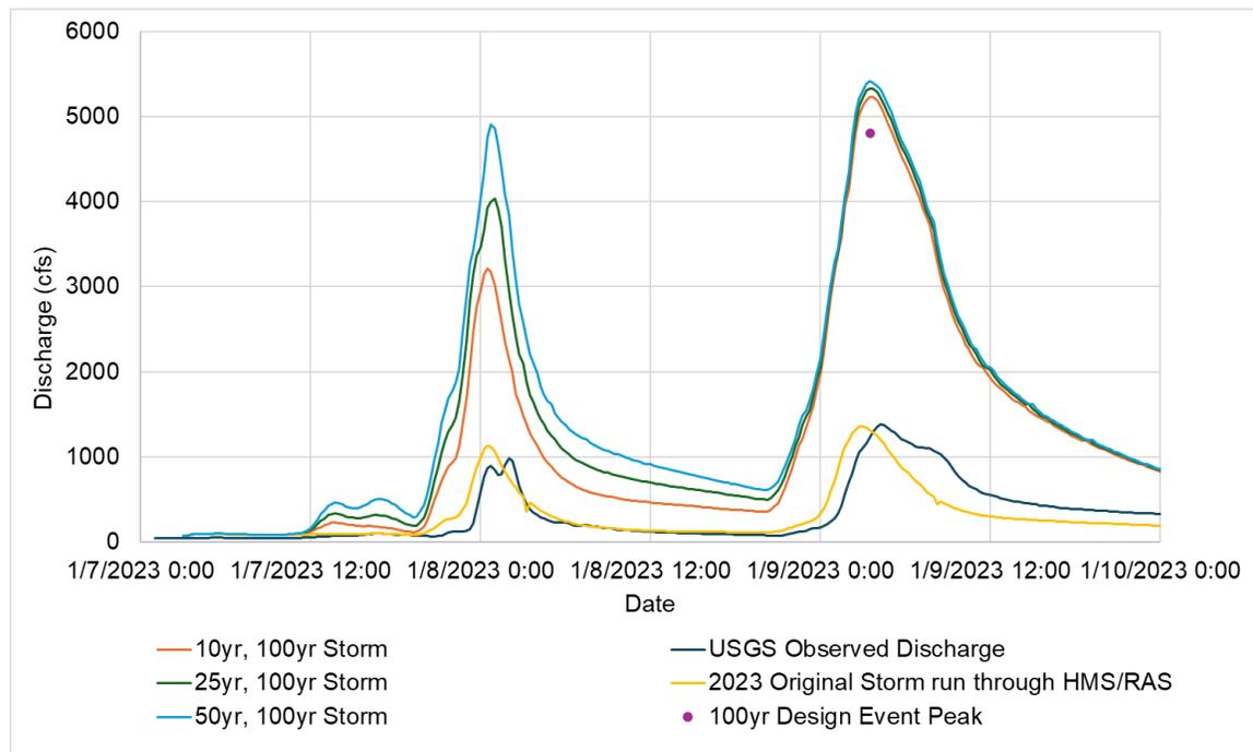
Figure 21. HEC-RAS hydrograph results at USGS Novato discharge gage 11459500
