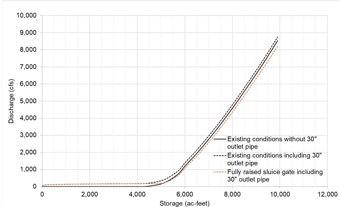
Figure 13. Storage-discharge curves for existing and proposed spillway
