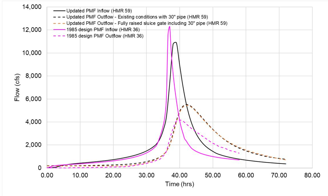
Figure 5. Comparison of inflow/ outflow hydrographs (PMF = 23.05" vs PMF = 31.28")
