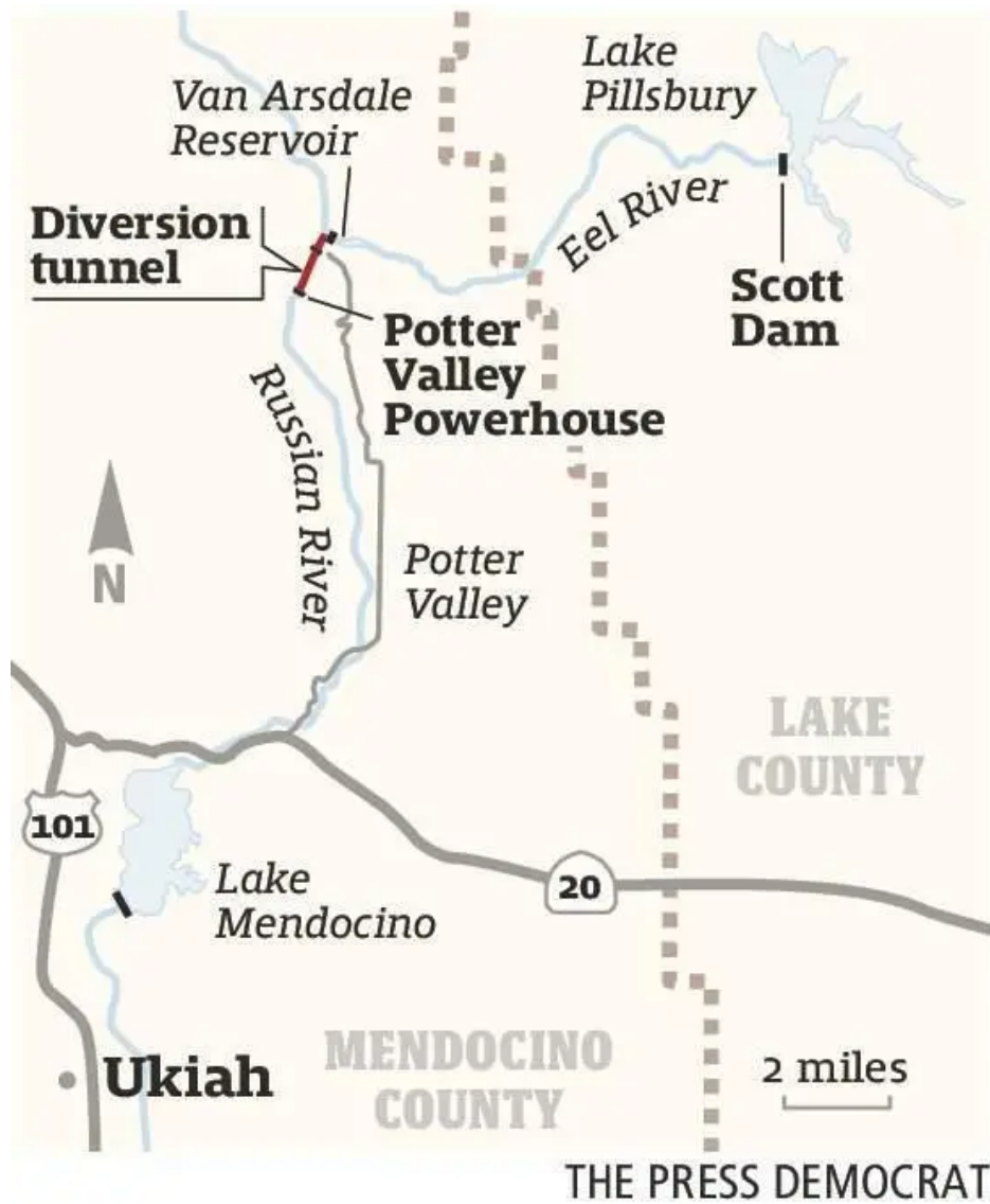
The Press Democrat This map shows the location of Scott Dam, impounding Lake Pillsbury, and Cape Horn Dam, creating Van Arsdale Reservoir, on the Eel River, the Potter Valley power plant, and the diversion tunnel that feeds the powerhouse and supplements flows in the East Fork of the Russian River. (The Press Democrat)
