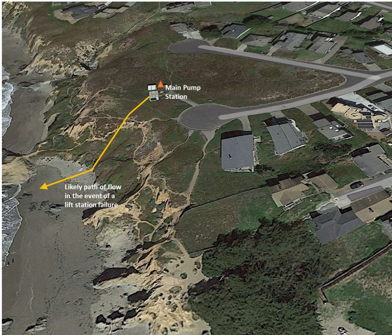
Figure 5-1. Main Lift Station Possible Spill Flow Path
